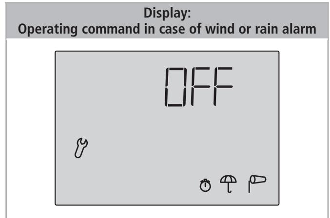
After the wind or rain alarm has been activated, the window is closed. The operating command for the connected drive mechanism either ends after 4 minutes or is permanently maintained as long as the alarm message exists.
