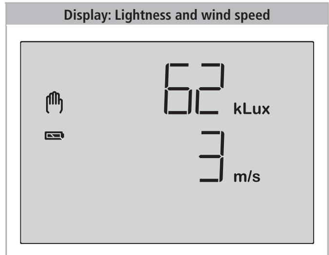
During the first approx. 90 seconds after the return of voltage at the weather station, the wind value is not displayed correctly (e.g. after a power fail or in case of a first start).
