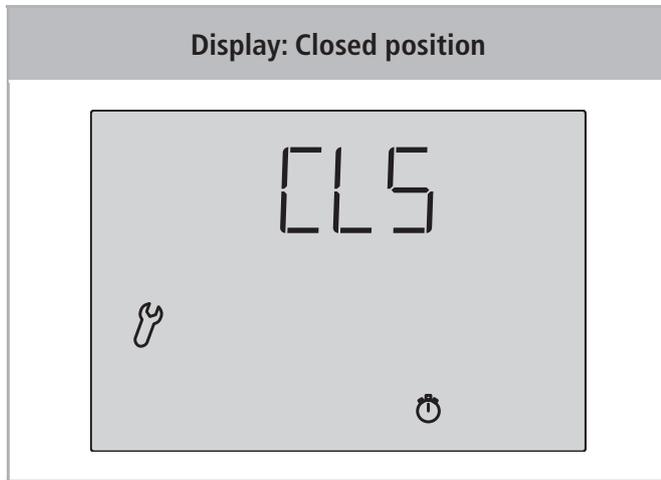
At first, completely close the window. Then press the **SET** key in order to access the next setting step.
