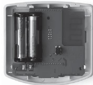
Close the housing by fitting the front panel with circuit board from above into the rear panel. The locking must engage with a clearly noticeable „click“.
