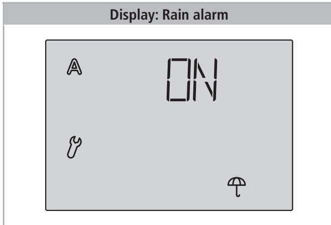
The rain alarm protects furniture and fixtures from damage. In case of rain, the window is automatically retracted and the manual operation is blocked.
