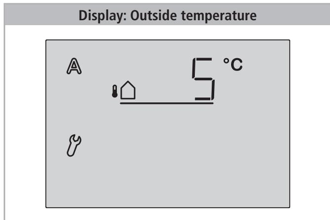
The outdoor temperature block keeps the window closed as long as the temperature is below the selected value. This means that in automatic mode, an opened window is closed and not opened again if the indoor temperature value (chapter A) is exceeded. Thus avoids energy losses during ventilation and protects plants from cold external air.
