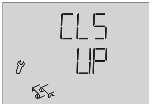
If the up and down connection cables have been mixed up when connecting the drive mechanism, this may be corrected in this step. First open the window a little bit for the rotational direction test. Check both arrow keys and make a setting in the display, whether the window closes again with  $\Delta$  or with  $\nabla$ .
