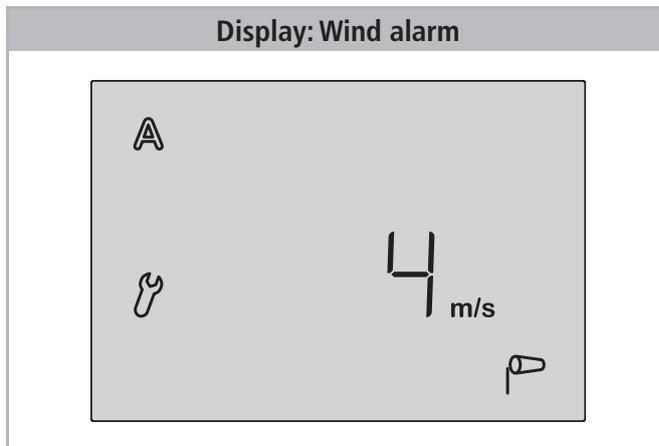
The wind alarm protects the window and furniture and fixtures from damage. If the indicated wind value is exceeded, the window closes and the manual operation is blocked. Wind speed is indicated in m/sec (meters per second).
